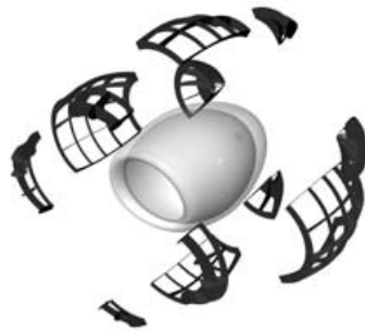
Engine - collaboration with Michel de Broin, digital fabrication and production management of sculpture, 3d modeling in Rhino, fabrication programming & documents, laser cut MDF and foam.
